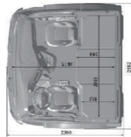
• Extended flat-roof narrow-body cab
